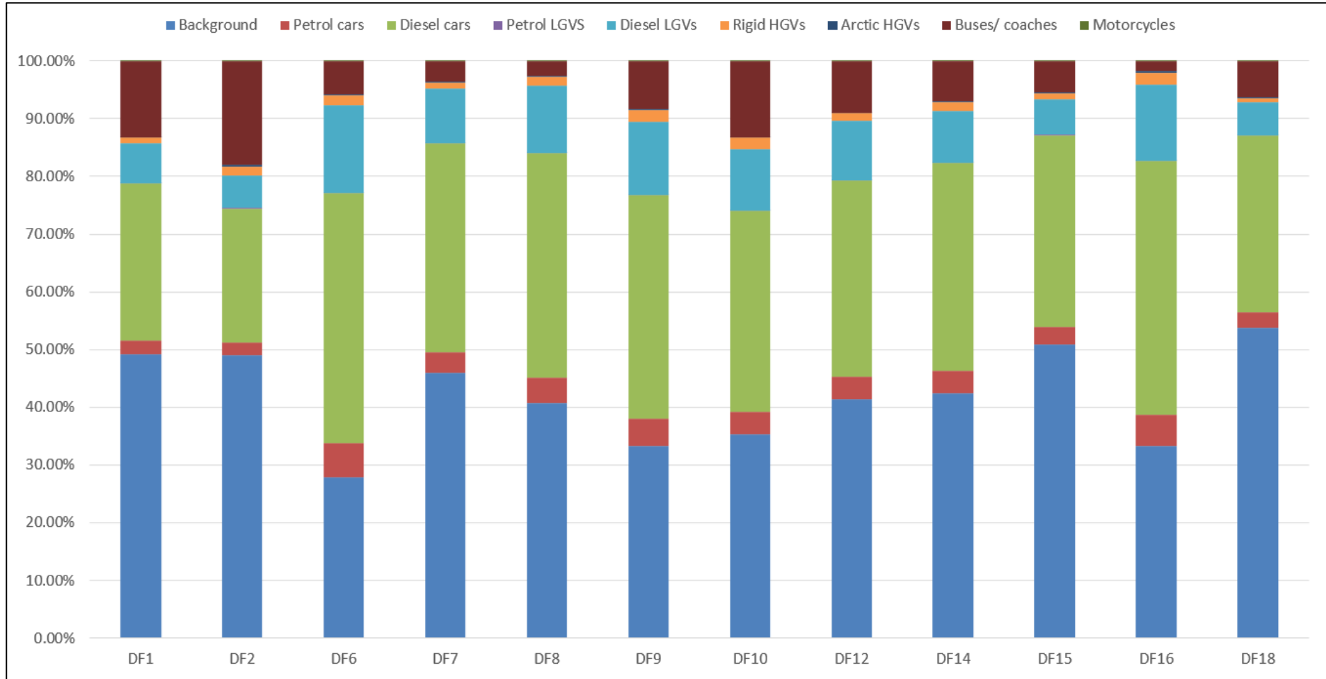
Figure 5: Stacked bar chart showing NOx source apportionment for all road transport and background for monitoring locations within Blackpool AQMA (%), for the baseline fleet, 2022
